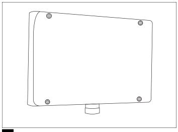
**Done**Cover the qaio power box up and securely tighten its screws.
