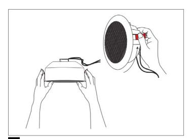
Pull the clip on both sides of the speaker. This will hold the speaker in place.
