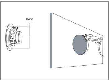
Cut an opening in the wall or ceiling where the speaker will be placed. Note that the size of the opening should be a little wider than the inner base of the speaker.
