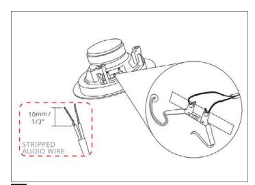
Flip the speaker to its back. Take your audio wires and strip them to about 10mm or 1/3 of an inch. Attach the stripped audio wires to the metal holes and secure them by soldering them.
