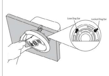
Tighten the dog-ear brackets by simply turning the screws inside the speaker's inner body. Use a philips head screwdriver to turn the screws slowly clockwise. The quickturn mounting system and frame will "sandwich" or clamp around the wall to hold the speaker securely in place.
